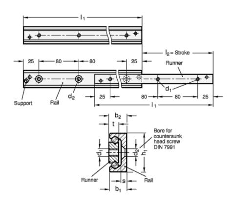
b1 = 21 b2 = 22 d1 = M8 d2 = 4.5 h1 = 43 L1 = 363 - 690s = 4.5t = 13.5Weight in (g) = 3590Weight in (g) = 3590s = 3590Weight in (g) = 3590Weight in (g) = 3590Weight in (g) = 3590Weight in (g) = 3590S = 3590S = 4.5S = 13.5
